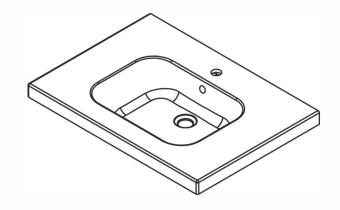
Faucet Holes are 13/8" Diameter Drain Holes are 113/16" Diameter Fireclay works best with a larger European drain Faucet Holes are available in 1 or 3
